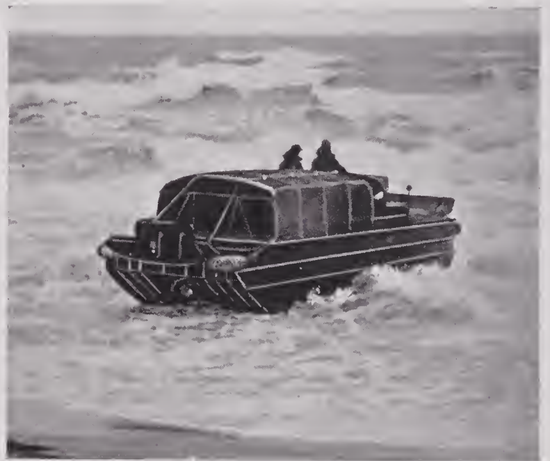
FIGURE 93. At official Provincetown demonstration, DUKW operates through moderate surf with waves ranging up to 6 feet in height.
